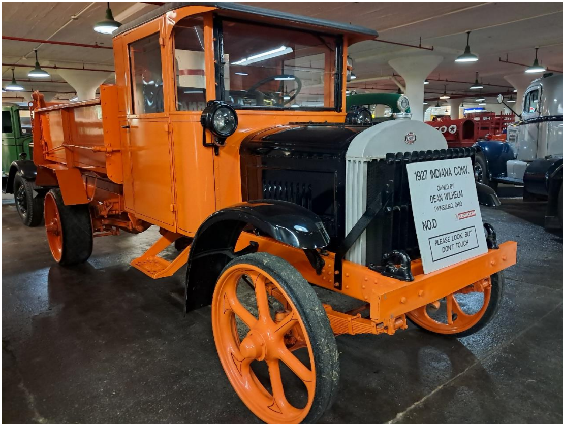
1927 Indiana Dump Truck with 3 ½ cubic yard body. The truck was stored in the 1930's with 16, 209 miles on its' odometer. Restored by Dean Wilhelm, at his shop - Dean's Truck Body, Inc. in Twinsburg, OH and displayed at NATMUS in Auburn, IN.
